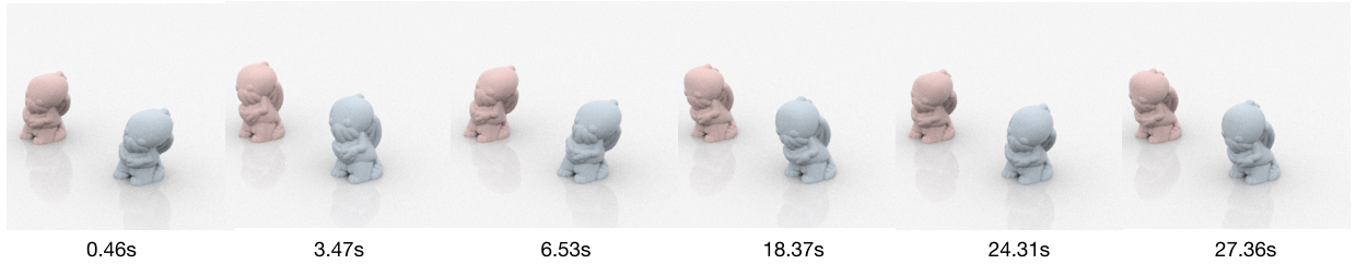
Fig. 18. Repetitive poking of a more complex geometry [126]. The object on the left (red) is the ground truth; the object on the right (blue) is the reduced-order simulation.
