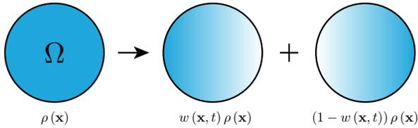
Fig. 2. **Blurred Density:** (Left) The reference domain  $\Omega$  of an object with density  $\rho(\mathbf{x})$ . Mass density is colored in blue. (Right) A partition of unity of the density mediated by a weight function  $w(\mathbf{x}, t)$ .
