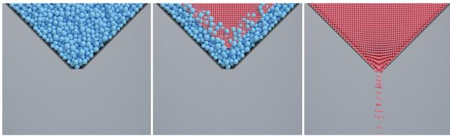
Fig. 12. Silo discharge (small orifice,  $r = 0.2$ ): A silo discharges grains with a discrete method (left), our hybrid method (middle), and a continuum method (right). Both the discrete and hybrid approach capture size-dependent clogging effects, and all flow from the orifice halts. The continuum simulation, in contrast, flows nonphysically.
