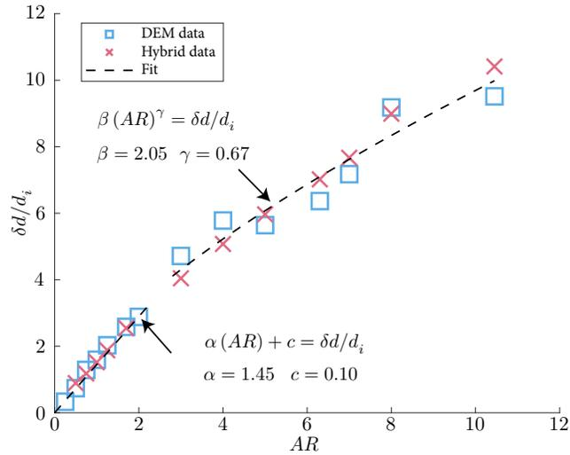
Fig. 6. Runout of a 2D granular column: Nondimensionalized runout distance,  $\delta d/d_i = (d_f - d_i)/d_i$ , vs aspect ratio,  $AR = h_i/d_i$ . Like DEM, our hybrid technique captures the two distinct regimes that Lube [2005] observed in experiments. We perform a linear fit in the low-AR regime, and a power-law fit in the high-AR regime.
